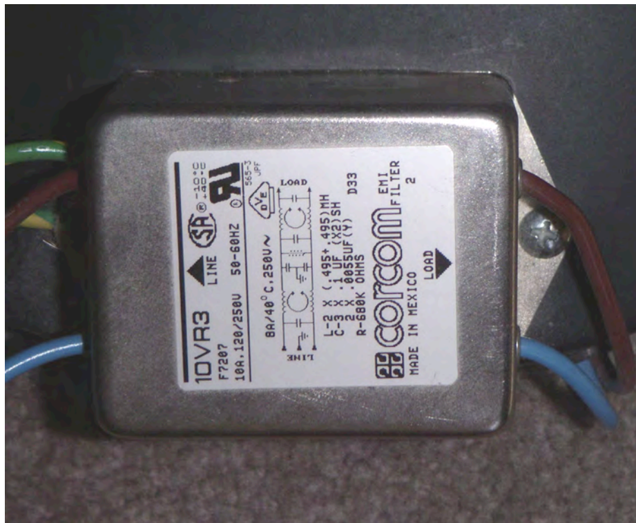
Figure 7: Corcom difference-mode EMI filter on base of QRN-generating lamp.
