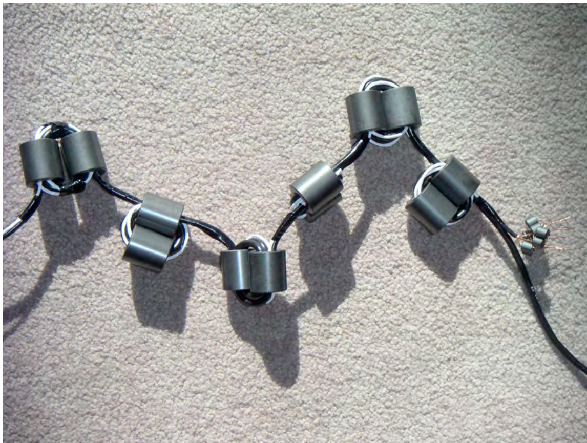
Figure 2: A series string of six binocular-core units like the one shown in Figure 1, on the parallel combination of an RG-58/U coaxial and a 5 \times AWG 26 tuner-control cable. Three of the six unit chokes were wound with three turns; and three have 2½ turns.
