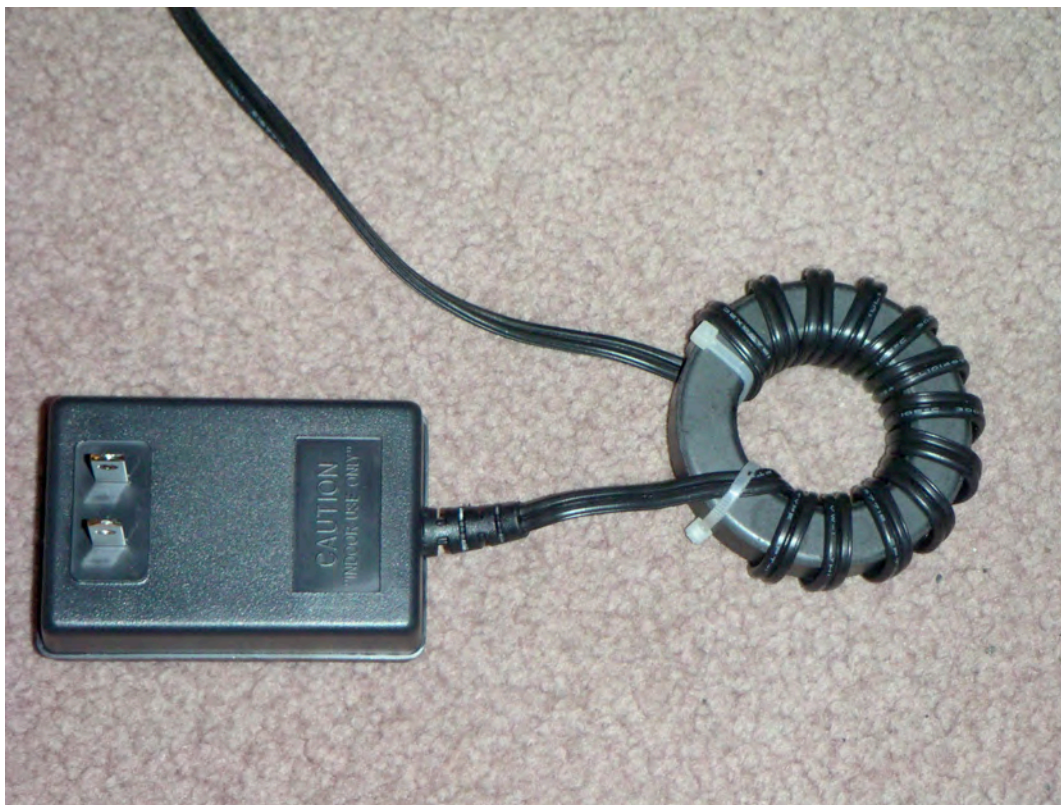
Figure 3: A wall-wart transformer for a modem, with a toroidal-core common-mode choke in its zip-cord, low-voltage, output cable. Near the other end of this cable, just before the modem, is another choke like this one.
