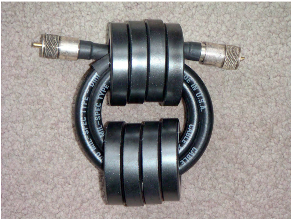
Figure 4: Common-mode choke for high HF power, formed by passing RG-213/U coaxial cable 3\frac{1}{2} times through a binocular core formed by two stacks of four Fair-Rite p/n 5943003801, mix-43, toroids. This choke's impedance exceeds 1\text{ k}\Omega from 1.8 through 18 MHz, dropping to 550\ \Omega at 30 MHz. One such choke should be installed at the antenna feedpoint, one at the amplifier output, and at least one other in-between.
